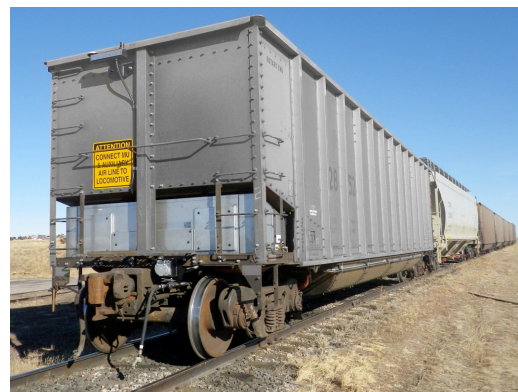
Figure 4: AutoPilot TORFM equipment mounted on a coal car
