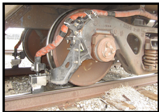
Fig 5: Friction Modifier Spray Application Nozzles
